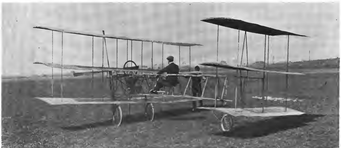
British Tri-plane That is Being Tested on Lea Marshes, by A. V. Row—It is Driven by Six-H.P. Jap Motor.
